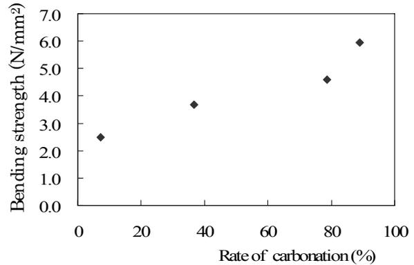
Figure 3. Relationship between Bending Strength and Rate of Carbonation
