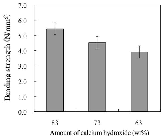
Figure 4. Relationship between the Bending Strength and the Amount of Calcium Hydroxide in the Board
