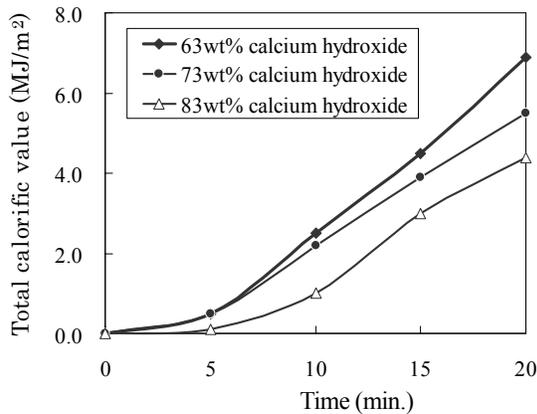
Figure 5. Total Calorific Value of the Board
