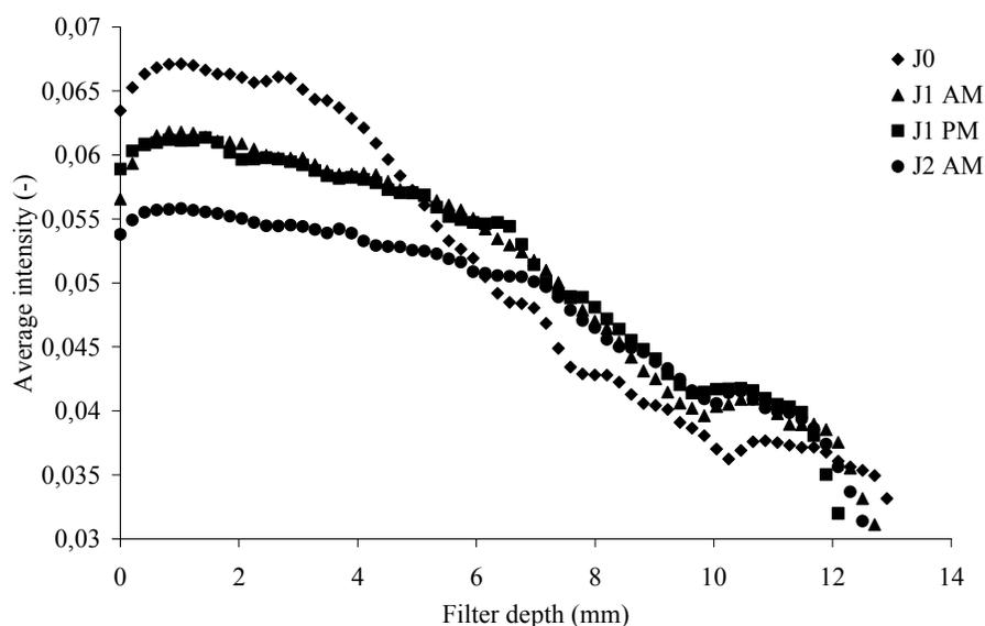
**Figure 3.** Re-distribution of  $\text{C}_6\text{H}_5\text{Cl}$  over time: concentration versus axial coordinate.
