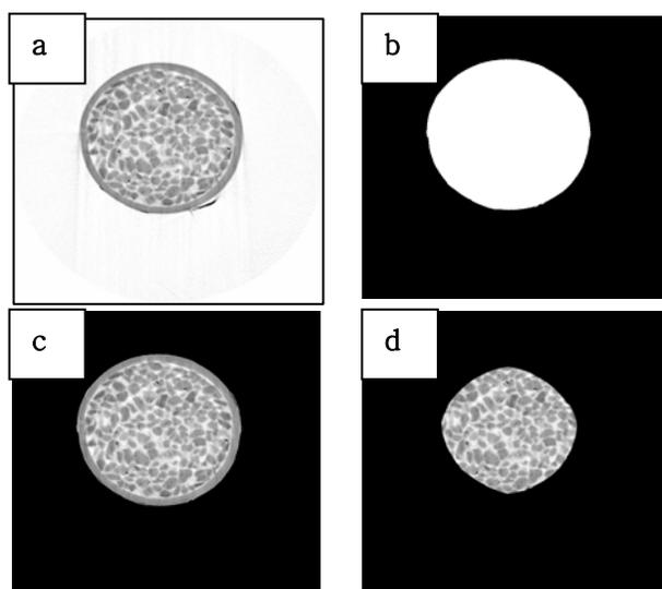
**Figure 1.** Example Image analysis processing - a. original cross section image b. binary mask c. elimination of background d. erosion of the image to exclude border effects.
