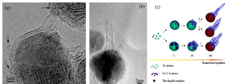
**Figure 3.** (a), (b) HRTEM images of the correlation between SWNTs, DWNTs and the attached catalyst particles, and (c) The diagram of the *localized liquid zone growth model at low temperature* for SWNTs and DWNTs produced by FCCVD method. (Ren WC, J. Nanosci. Nanotechnol. & J. Phys. Chem. B 2006)
