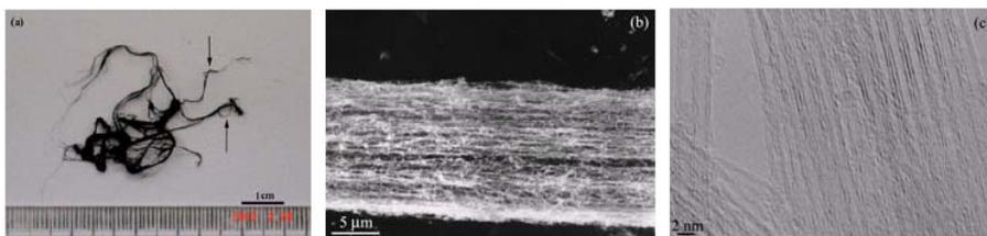
Figure 2. Optical photo, SEM and HRTEM images of aligned DWNT ropes. (Ren WC, J. Phys. Chem. B 2005)
