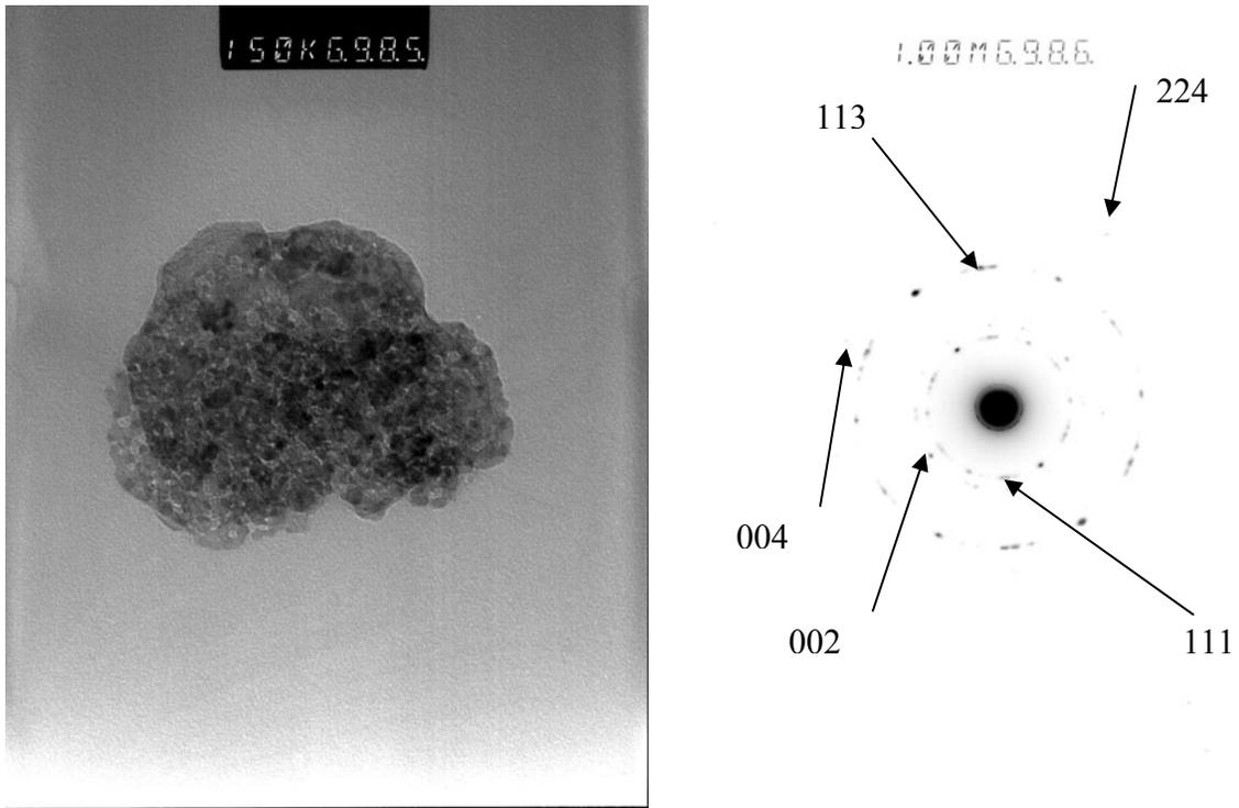
**Figure 2.** Cubic nanodiamonds. Diffraction pattern shows monocystal spots (right).
