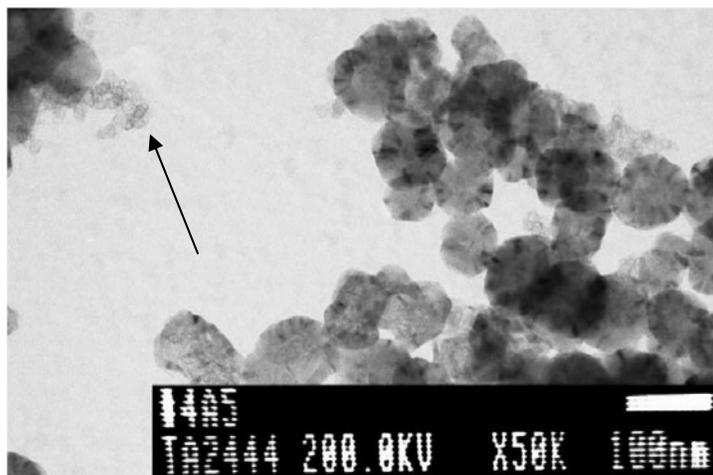
**Figure 1.** Along with SCNPs a cluster of giant fullerenes of 5 nm is shown by the arrow in the left upper corner.
