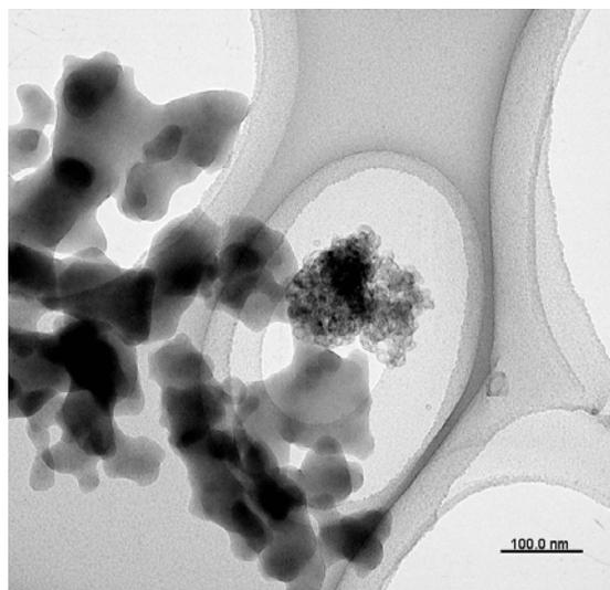
**Figure 4.** Amorphous carbon along with giant fullerenes.
