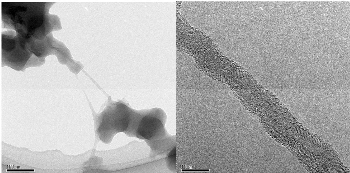
**Figure 3.** Carbon nanotubes are seen on the background of amorphous carbon. One of the nanotubes is multiwalled (HRTEM image on the right), the other - amorphous.
