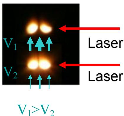
**Figure 5.** Photographic images of the reaction zones for two flow velocities. Blue arrows indicate flow direction and parabolic profile; red arrows indicated the laser beam size and direction for the two cases.
