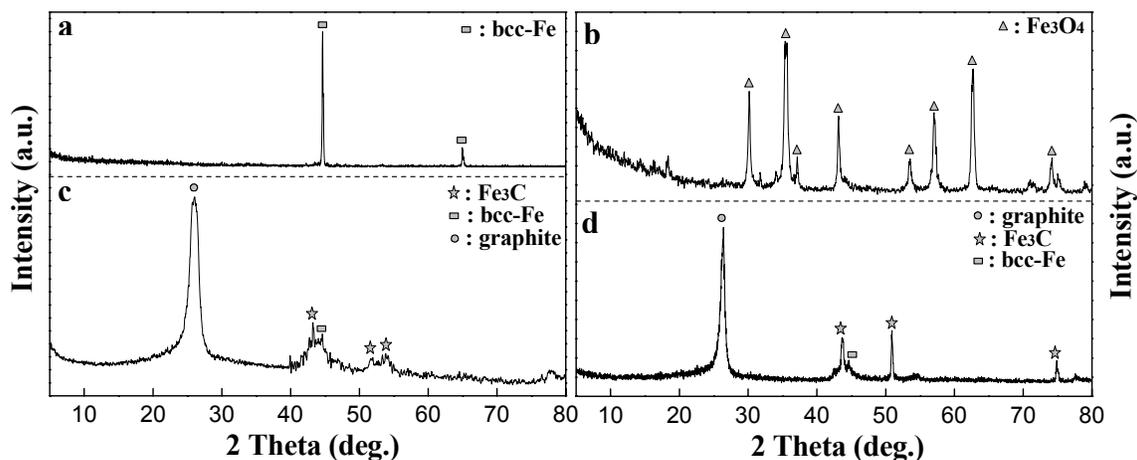
**Figure 1.** XRD patterns of the catalysts calcined under (a) H<sub>2</sub> and (b) N<sub>2</sub>. (c) and (d): XRD patterns of the carbon samples deposited over Cat<sub>H</sub> and Cat<sub>N</sub>.
