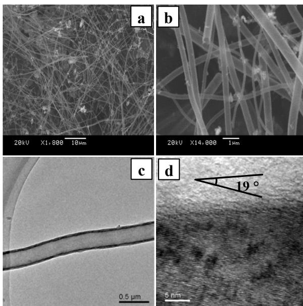
**Figure 3.** SEM images (a and b) and TEM results (c and d) of the fishbone-type CNTs
