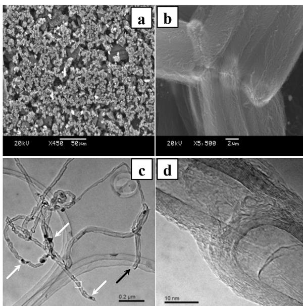
**Figure 2.** SEM images (a and b) and TEM results (c and d) of the bamboo-shape CNTs.
