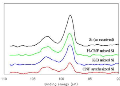
**Figure 2.** XPS analysis of Si element. a) Si(as received) b) CNF synthesized Si, c) H-CNF mixed Si, d) K/B mixed Si.
