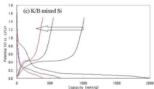
**Figure 3.** Charge-discharge profiles until 3 cycles. a) CNF synthesized Si, b) H-CNF mixed Si, c) K/B mixed Si.
