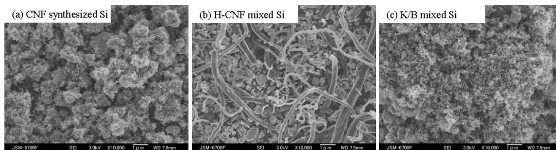
**Figure 1.** SEM images of a) CNF/Si composite, b) H-CNF mixed Si; c) K/B mixed Si, respectively.
