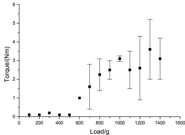
Figure 2. Effect of tool load on torque for unoxidised IM1-24 graphite. Rotational speed 50 rpm; error bars show  $\pm 2$  standard deviations.
