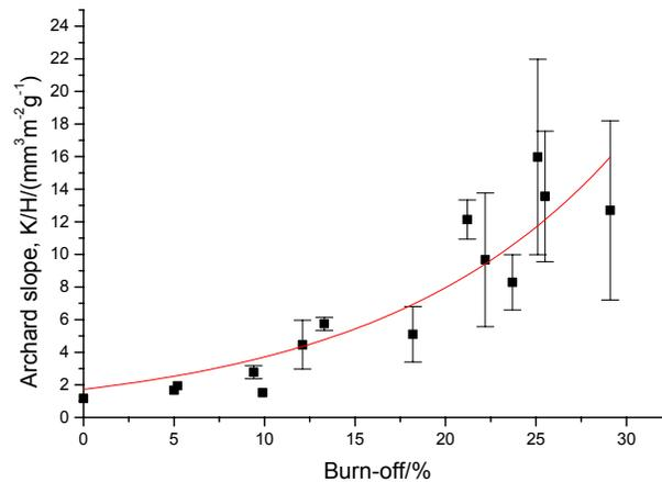
Figure 5. Variation of the Archard slope  $K/H$  with extent of oxidation of IM1-24 graphite. Error bars are  $\pm 2$  standard deviations
