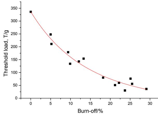
Figure 6. Variation of cutting threshold,  $T$ , with extent of oxidation of IM1-24 graphite.
