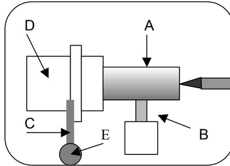
Figure 1. Apparatus for measuring dynamic friability of graphite (schematic).
