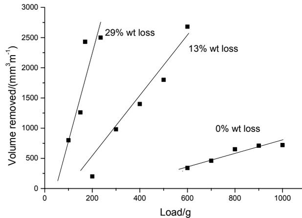
Figure 4. Effect of oxidation upon the wear of IM1-24 graphite. Rate of rotation = 50 rpm
