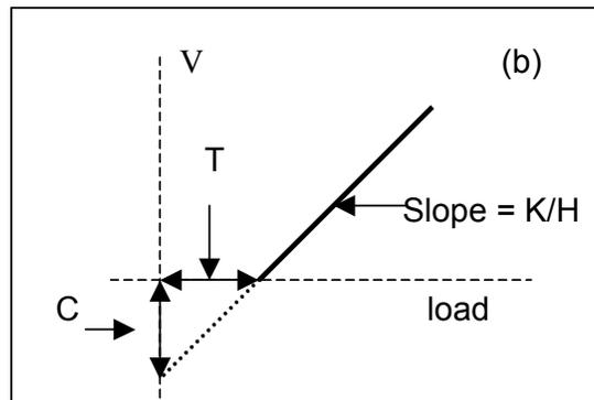
Figure 3. (a) Effect of tool load on the volume of graphite removed per unit sliding distance,  $V$ . Rotational speed, 50 rpm; error bars are 2 standard deviations. (b) Fit of Fig 3(a) to the modified Archard Equation, see text.
