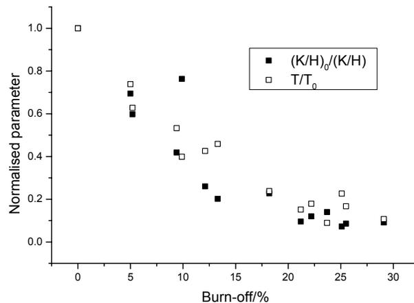
Figure 7. Effect of oxidation upon the normalised inverse Archard slope  $(K/H)_0/(K/H)$  and normalised threshold load,  $T/T_0$ .
