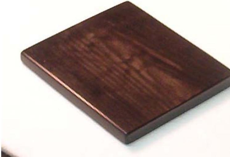
**Figure 3.** Carbon-polymer composite plate made from yellow pine.
