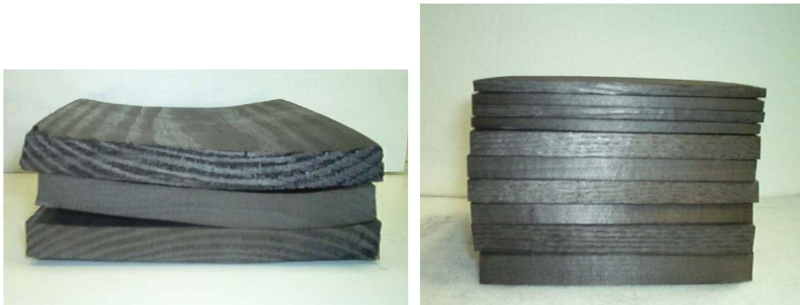
**Figure 2.** Carbonized wood specimens processed without boundary restraint left, and with on right. Sample size of approximately 1.5 x 12 x 12 cm.
