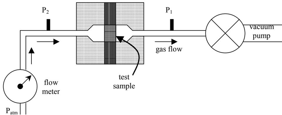
**Figure 1.** Schematic of permeability set-up for wood and carbonized wood.
