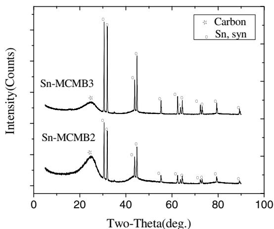
**Fig.3** The XRD patterns of Sn-MCMB carbonized at 1000°C
