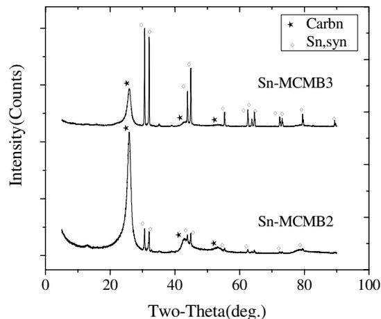
**Fig.4** The XRD patterns of Sn-MCMB carbonized at 1800°C
