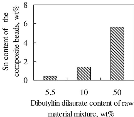
**Fig.1** Sn content of composite microbeads changes as a function of dibutyltin dilaurate content of raw material
