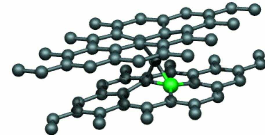
Figure 1. Self-interstitial pinned at a boron impurity
