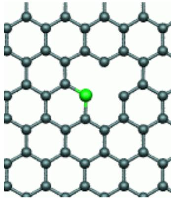
Figure 2. Lattice vacancy pinned at a boron impurity
