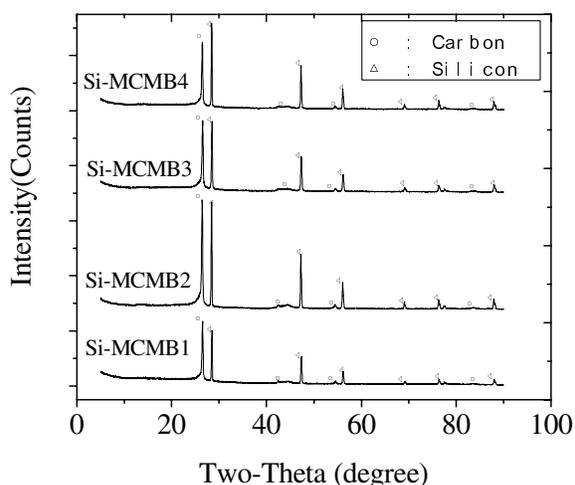
**Fig.1.** The XRD patterns of Si-MCMB composites
