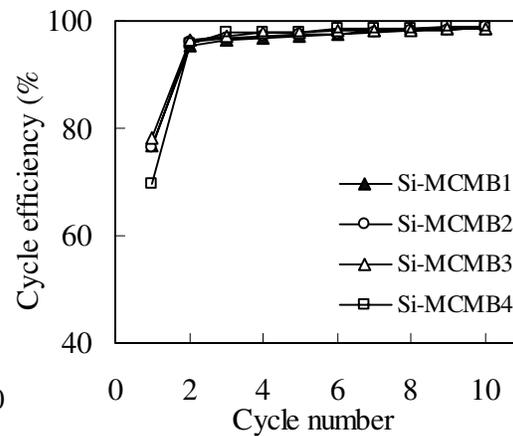
Fig.4. The cycle performance of Si-MCMB composites
