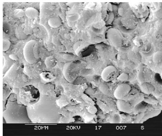
**Fig.2.** The SEM image of Si-MCMB3 composites
