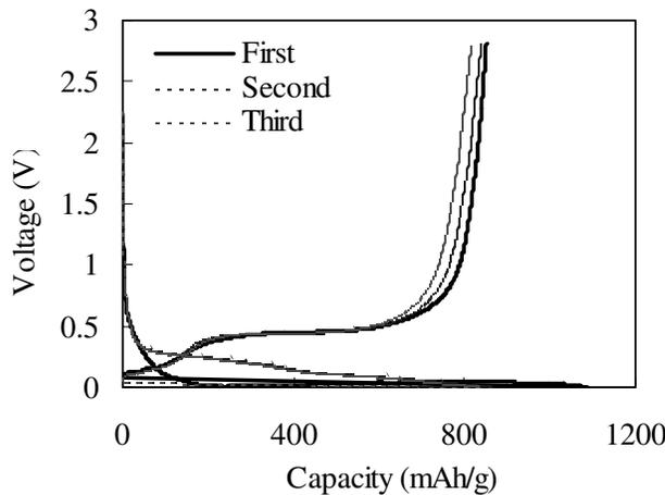
Fig.2. The discharge and charge curves of Si-MCMB3 composites
