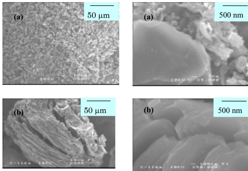
Fig.1 SEM photograph of activated carbon derived from AR resin (a) and needle coke (b)
