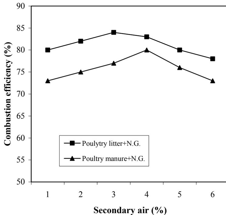
Figure 3 Carbon combustion efficiency as function of secondary air (Excess air is 25%, secondary air height is 0.65m)
