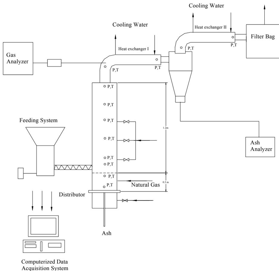
Figure 1 the schematic diagram of the SFBC laboratory scale waste disposal system
