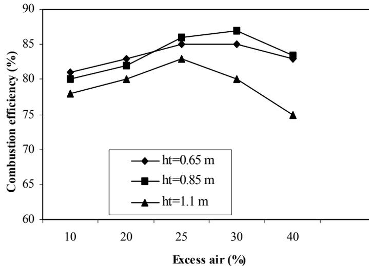
Figure 5 Carbon combustion efficiency as function of secondary air injection layer (Poultry litter +N.G., Secondary air 25%)
