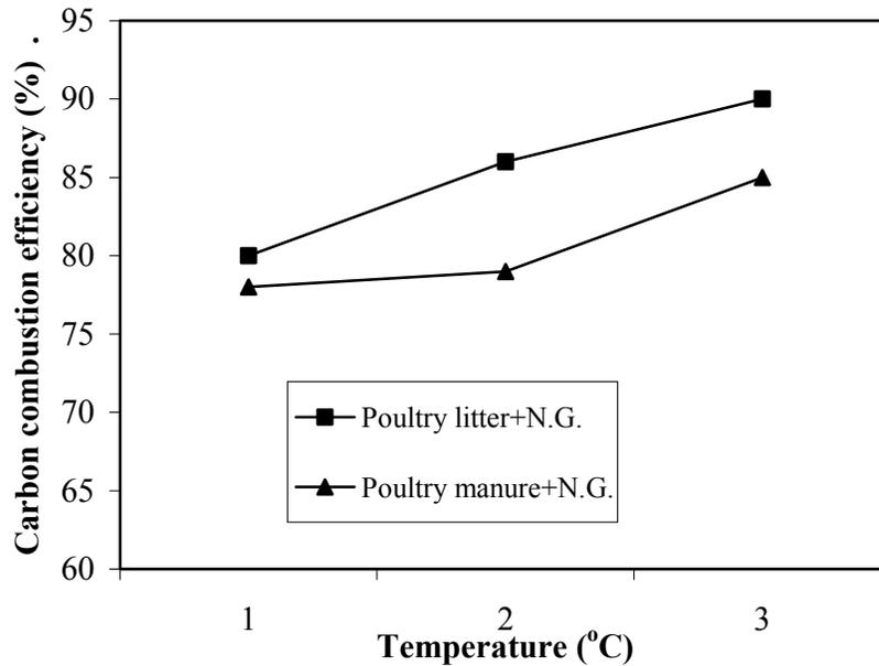
Figure 2 Effect of temperature on the carbon combustion efficiency
