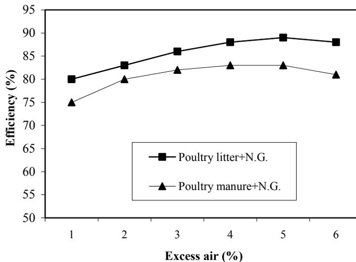
Figure 3 Carbon combustion efficiency as function of excess air ratio (Secondary air 20%, with 0.85m injection height)
