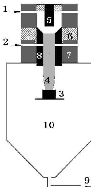
**Fig. 1** Schematic drawing of the setup for making carbon nanotubes from pitch under arc jet plasma conditions; (1) cathode working gas, (2) anode working gas, (3) graphite boat, (4) arc plasma torch, (5) cathode, (6) insulator, (7) cooling water, (8) anode, (9) vent, (10) reactor.
