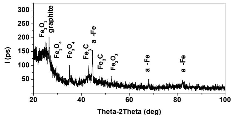
**Fig. 2** Typical XRD pattern of as-synthesized CNTs
