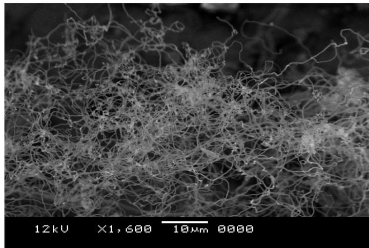
**Fig. 3** Typical SEM image of CNTs from mesophase pitch under arc-jet plasma conditions.
