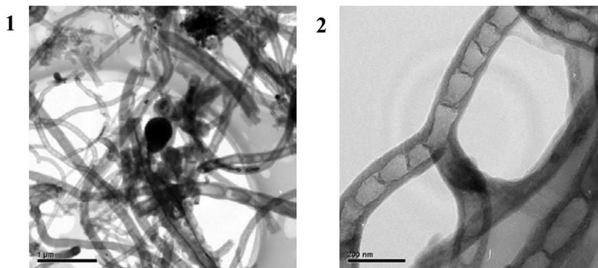
**Fig. 4** TEM images of CNTs; (1) TEM image of as-synthesized CNTs; (2) a typical TEM image of CNTs, showing bamboo-like characteristics of the tubes.
