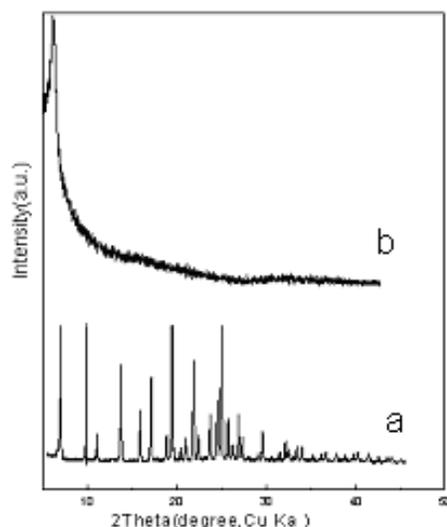
Fig. 1 The XRD patterns of Y zeolite (a) and the resultant carbon (b).
