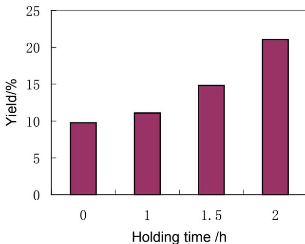
Fig. 4 The yield of carbons vs. the holding time in soakage under 1.3 MPa N<sub>2</sub>
