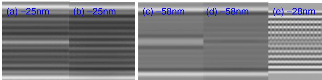
Figure 1 Simulated images of MWCNT without 0.3nm nanotube at the core (a, c) and with 0.3nm nanotube core (b,d). Simulated image under 1200keV condition is shown in (e)
