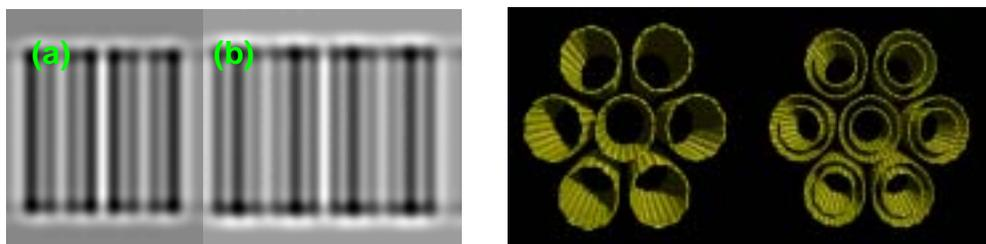
Figure 2 Simulated images of SWCNT bundle and DWCNT bundle. Can you tell which is which? (a) is the SWCNT bundle, and (b) is the DWCNT bundle.
