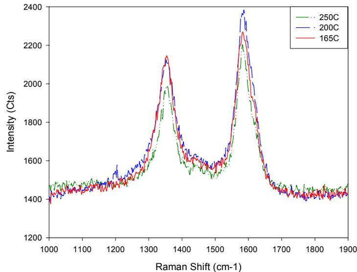
Fig.3. Raman spectrum of carbon nanotubes produced at different injection temperatures.
