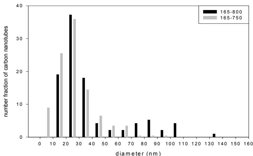
Fig. 1. Diameter distributions of carbon nanotubes produced at different reaction temperatures and 165° of injection temperature.
