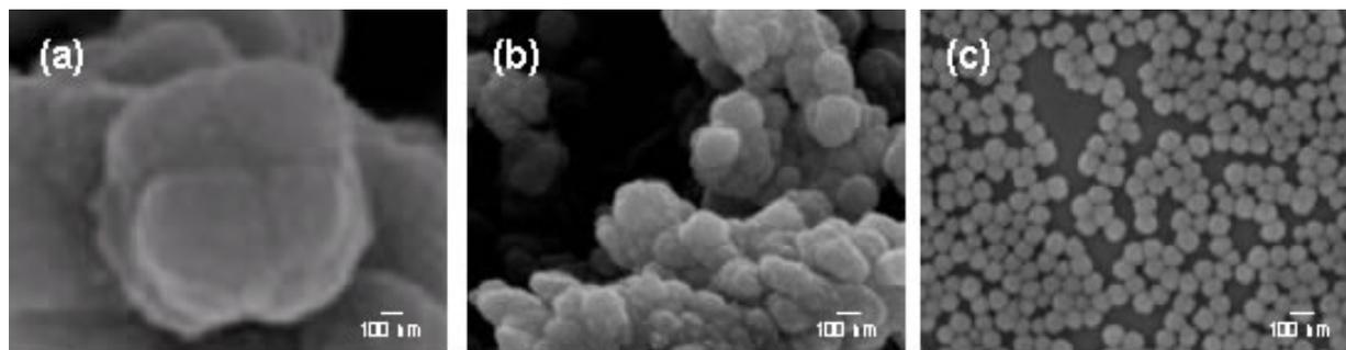
Figure 1. SEM micrographs of PPy particles by bulk polymerization method (a), and the controlled monomer feeding rate method without PVA stabilizer (b) and with stabilizer (c).
