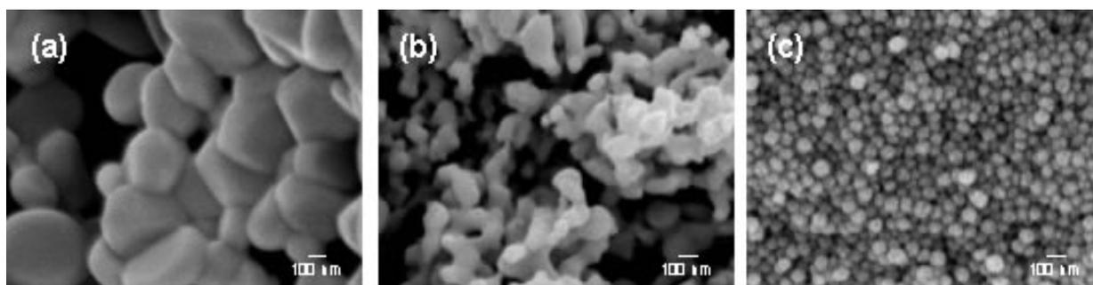
Figure 2. SEM micrographs of carbonized PPy particles by bulk polymerization method (a), and the controlled monomer feeding rate method without PVA stabilizer (b) and with stabilizer (c).
