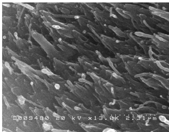
Figure 3. SEM micrograph of a fracture surface of a 5 wt.% mispMWNT/PAN composite fiber showing the 'balling-up' effect on the nanotube surface
