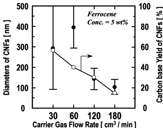
Fig. 2 Effects of carrier gas flow rate on CNF diameter and yield
