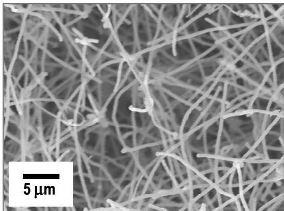
Fig. 1 SEM image of typical CNFs obtained in this work
