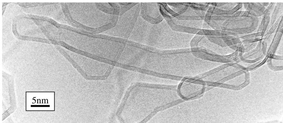
Figure 2. Structure of fullerene soot following high temperature heat treatment in a graphite furnace.
