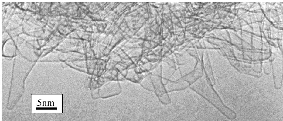
Figure 1. Tube-like structures observed in fullerene soot following high temperature heat treatment in an electron gun.
