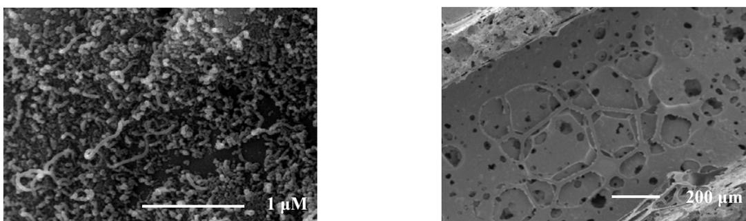
Figure 2. SEM images of prepared carbon coatings. a:carbon fibers, b:sucrose
