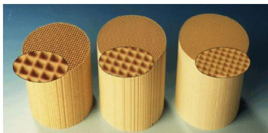
control systems where low pressure drop and high surface area are paramount [8], are an interesting alternative for conventional support materials in heterogeneous catalysis. These porous macro structured supports consist of small square channels on which a thin layer of active material can be applied [9].
