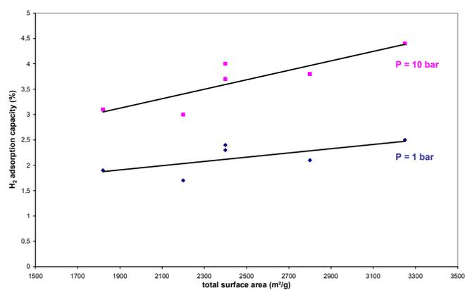
Figure 1 : H<sub>2</sub> adsorption capacity versus total surface area
