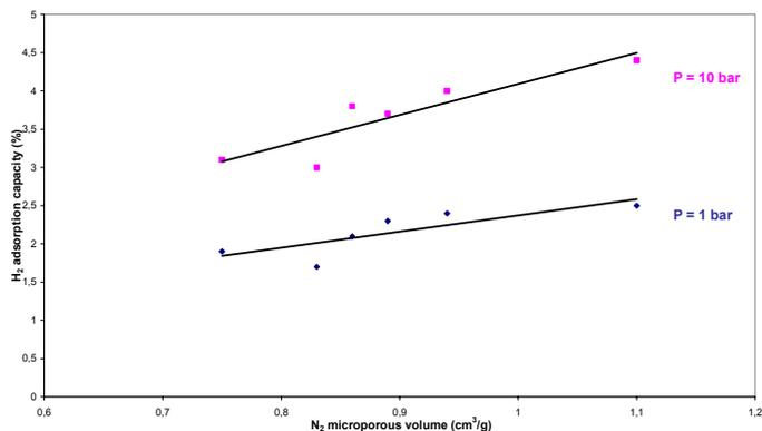
Figure 2 : H<sub>2</sub> adsorption capacity versus N<sub>2</sub> micropore volume (D < 2 nm)
