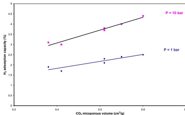
Figure 3 : H<sub>2</sub> adsorption capacity versus CO<sub>2</sub> micropore volume (D < 0,7 nm)
