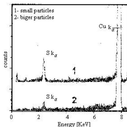
Fig. 2. The EDAX spectra showing sulfur concentrations for particles of different sizes
