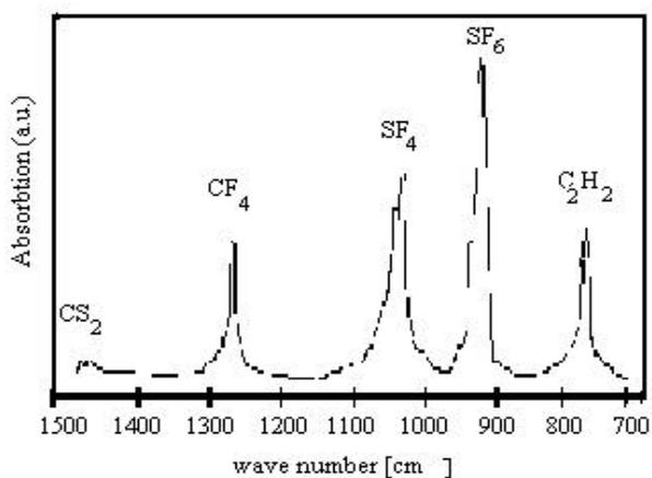
Fig. 1. The IR spectrum of exhaust gases in a run using C<sub>2</sub>H<sub>2</sub>/SF<sub>6</sub> mixture
