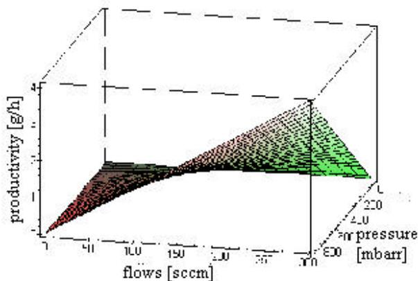
Fig. 6. The productivity (g/h) of carbon powder vs. pressure and gas-flow
