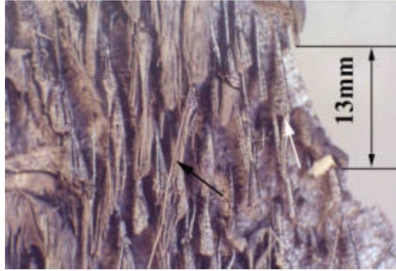
Fig 2 macroscopic image of quasi-VGCF (shown by white arrow) and VGCF (shown by black arrow)
