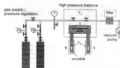
Figure1 CAHN balance of the gravimetric methane
