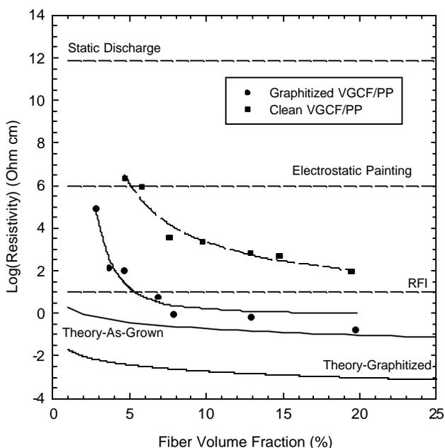
Figure 1. Approximate resistivity upper bound required for several applications, compared to electrical resistivity values measured for graphitized VGCF and clean VGCF in polypropylene.
