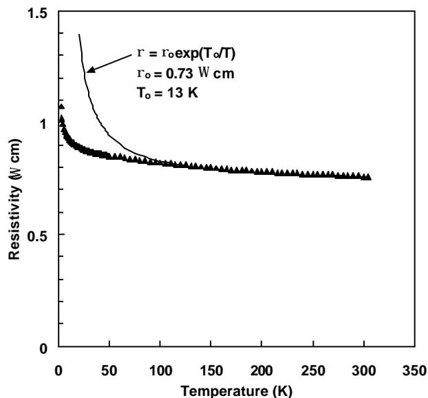
Figure 2 Resistivity of an 8 vol% graphitized fiber/PP composite vs temperature. Solid curve is a least squares fit to the resistivity equation shown in the plot.
