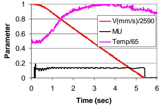
Figure 5. Temperature, velocity and mu during simulated taxi stop.
