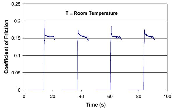
Figure 9. Friction test data from c/c composite at room temperature, 4 passes (24°C).
