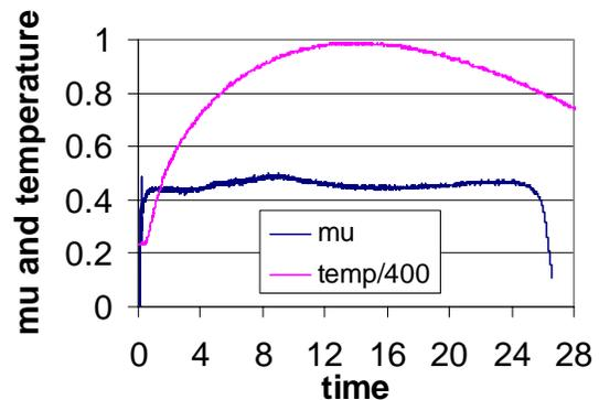
Figure 6. Temperature and mu during simulated landing stop.
