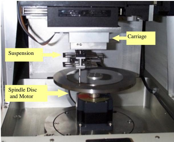
Figure 4. Carriage, suspension and spindle assembly of the pin-on-disc tribometer.
