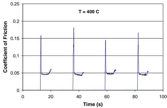
Figure 11. Friction test data from c/c composite at 400°C, 4 passes.
