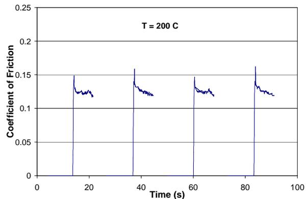
Figure 10. Friction test data from c/c composite at 200°C, 4 passes.
