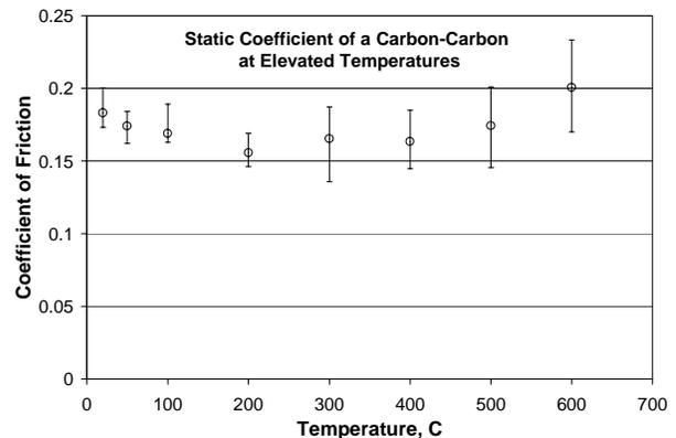
Figure 13. Static friction coefficient of c/c as a function of temperature.
