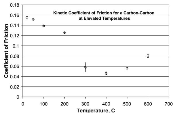
Figure 14. Kinetic friction coefficient of c/c as a function of temperature at low speed.
