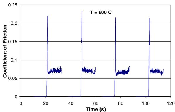
Figure 12. Friction test data from c/c composite at 600°C, 4 passes.
