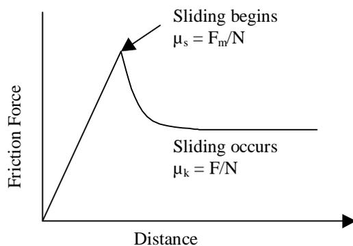
Figure 2. Schematic showing change from static to kinetic friction.
