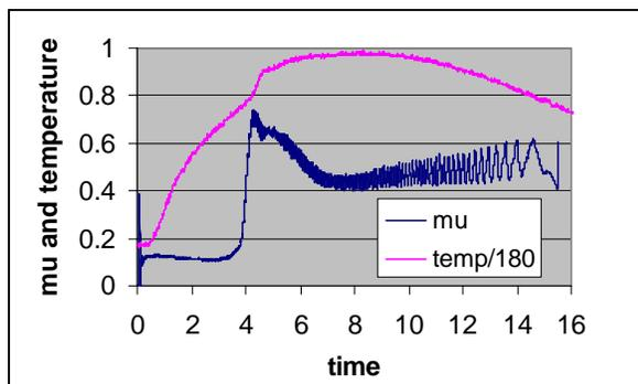
Figure 1. Dynamometer stop shows abrupt increase in friction when near-surface temperature exceeds 130°C for C/C composites. Cause: moisture desorption transition.
