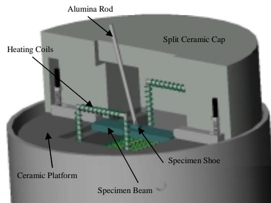
Figure 3. Schematic of high temperature furnace for friction tests in reciprocating mode.
