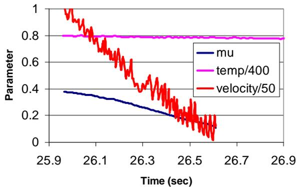
Figure 7. Velocity, temperature and mu at the end of a landing stop. (velocity in mm/s)
