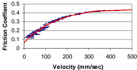
Figure 8. Velocity dependence of mu at the lowest speeds of a landing stop, temperature at ~320°C.
