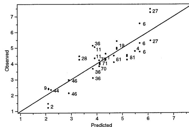
**Figure 2.** Observed versus predicted  $1/k'$  for initial break-through on BPL carbon as received.
