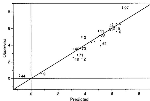
**Figure 1.** Observed versus predicted  $1/k'$  for initial break-through on prehumidified BPL carbon.
