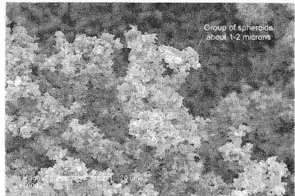
Figure 1: Shows coating deposited with notch. Coating formed using 10 minutes of *spheroid conditions*.
