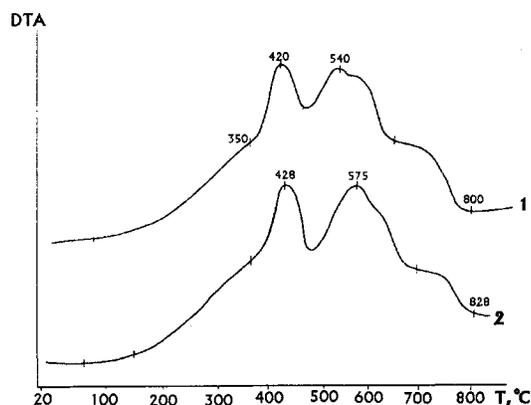
**Figure 1.** DTA curves of the composite materials: 1-EPAN, 2-EPAN with shungite-filler
