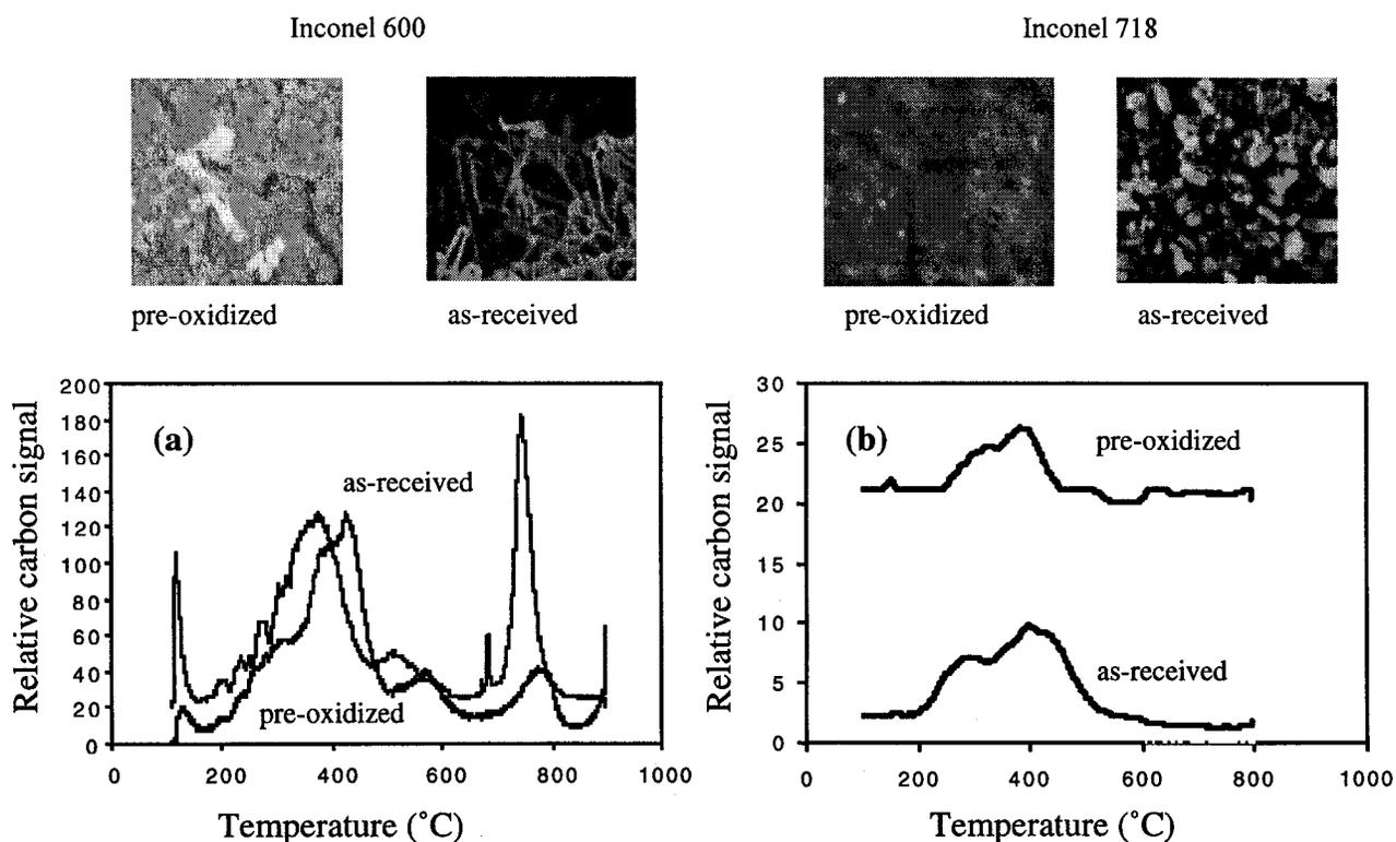
Figure 1. Temperature-programmed oxidation profiles and SEM micrographs for deposits on as-received and pre-oxidized coupons of Inconel 600 (a), and Inconel 718 (b).
