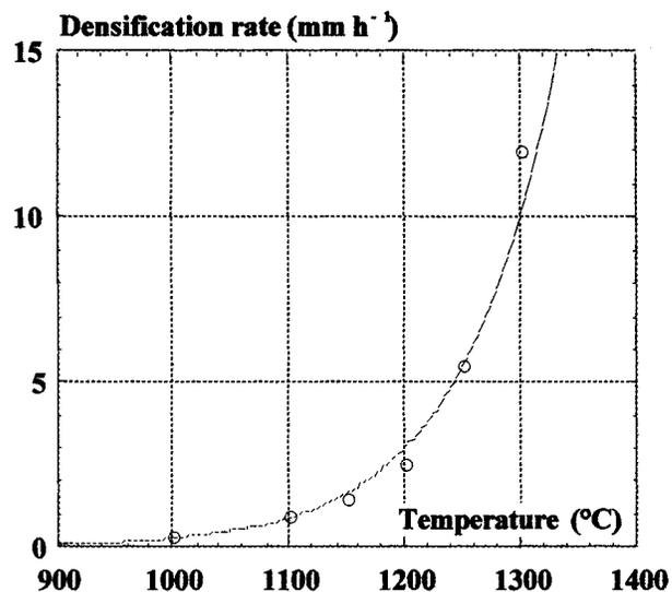
Fig. 3: Densification of a carbon felt (from cyclohexane)
