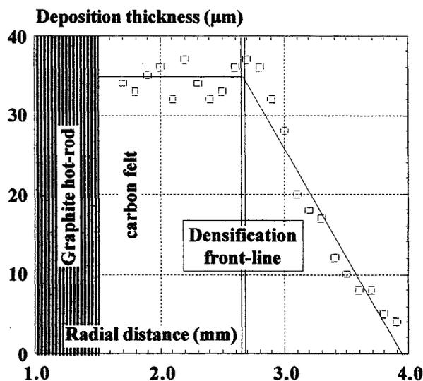
Fig. 2: Radial densification profile (from cyclohexane, 30' at 1250°C)
