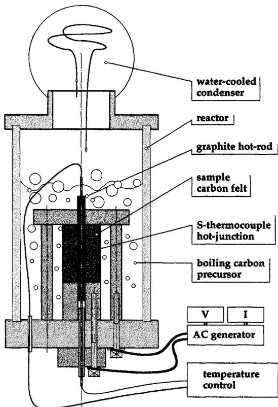
Fig. 1: Experimental set-up
