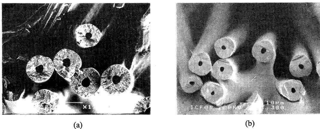
**Figure 2.** SEM photographs of hollow mesophase (a) and isotropic (b) pitch-based carbon fibers.
