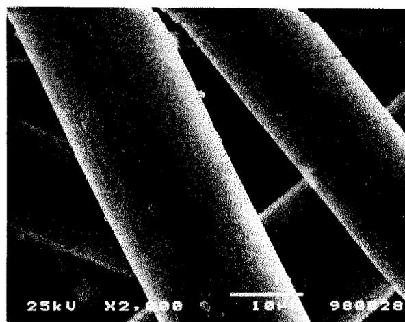
Fig. 2. SEM micrograph of Cu treated ACF.
