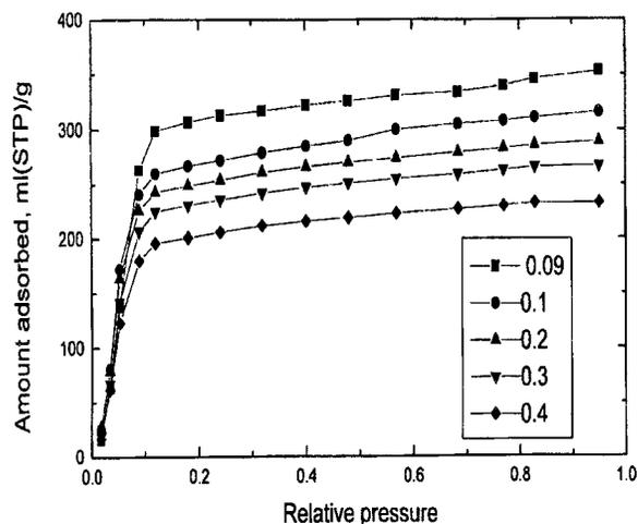
Fig. 1. Adsorption isotherm of nitrogen on the Cu treated ACF.
