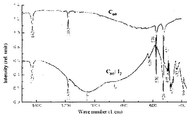
Fig.1. IR spectra of pure fullerene and iodine intercalated fullerene film.
