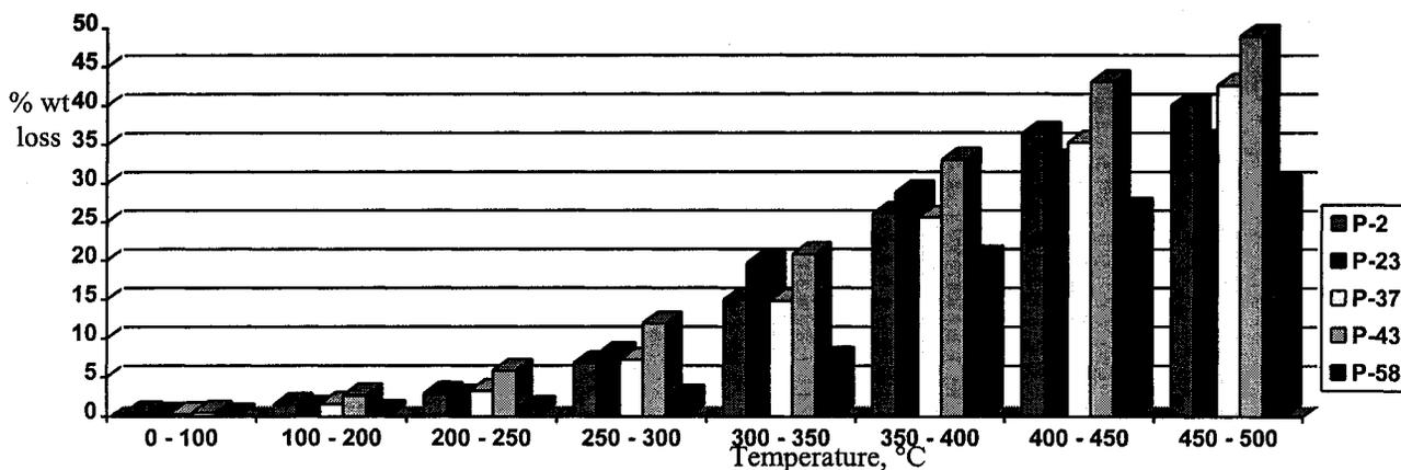
**Figure 1.** % wt loss of material as a function of temperature as obtained from TG thermograms.
