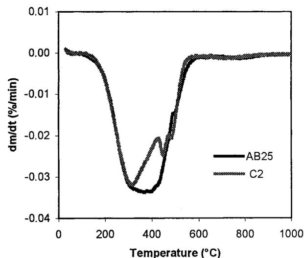
**Figure 1.** DTG curves of a thermally treated pitch and an air-blown pitch.
