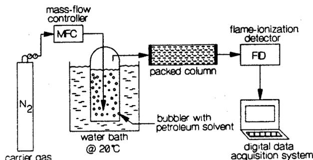
Figure 1. Apparatus for screening adsorbents.
