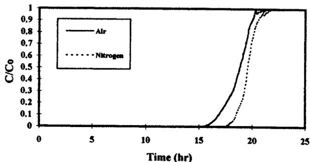
**Figure 2.** Xtrusorb-800 Breakthrough Curve. Carrier flow rate = 350 cc/min
