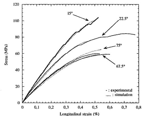
Figure 4 : Comparison of predicted and experimental stress-strain curves for various off-axis tensile loading conditions (15°, 22.5°, 67.5°, and 75° with respect to direction 1)
