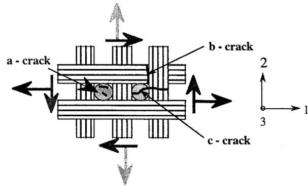
Figure 2 : Schematic diagram summarizing the three families of cracks detected during the tensile and the shear tests
