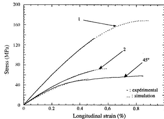
Figure 3 : Comparison of computations with the experimental stress-strain curves for damage parameters identification : on-axis (directions 1 and 2) and off-axis (45° in the plane of the plies) tensile tests
