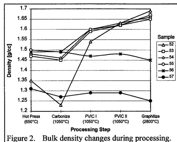
Figure 2. Bulk density changes during processing.
