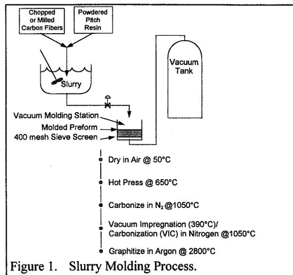
Figure 1. Slurry Molding Process.
