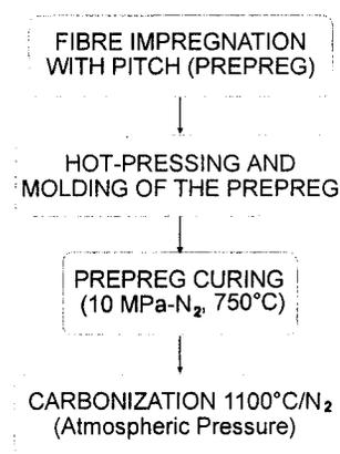
Figure 1. Diagram of the laboratory process of composites preparation.
