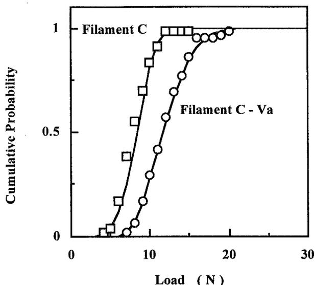
Figure 1. Tensile load distribution of carbon filaments
