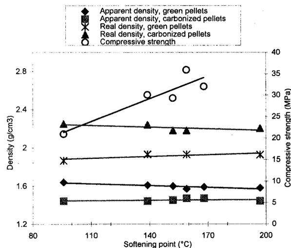
Figure 1-. Densities and mechanical properties of pellets.
