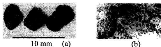
Fig.1. Carbon granules (a) and their surface picture (b).
