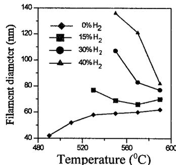
Fig. 3. Temperature dependence of the filament diameter.
