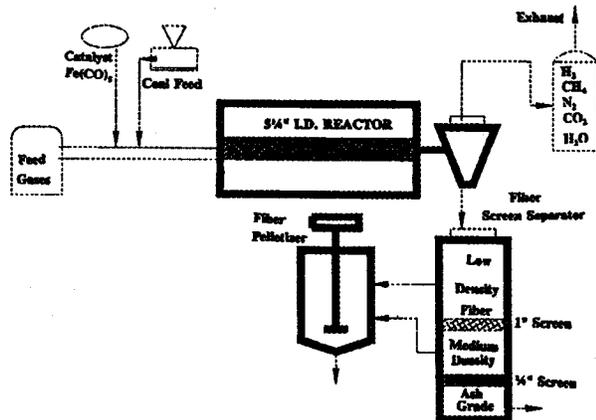
Figure 1. VGCF Process Schematic
