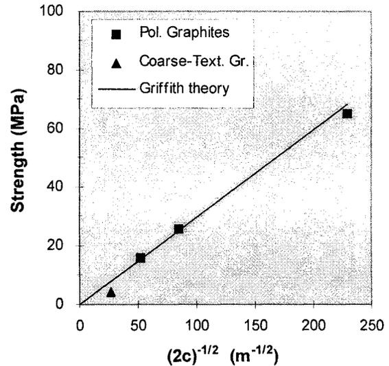
**Figure 1.** Tensile strength ( $\sigma_{TS}$ ) of the graphites as a function of  $(2c)^{-1/2}$ . The theoretical curve was obtained from eqn (1) with  $E = 11.0 \text{ GPa}$  and  $\gamma_{app.} = 6.4 \text{ Jm}^{-2}$ .
