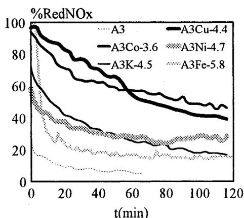
Figure 2. Isothermal reaction curves at 300°C.
