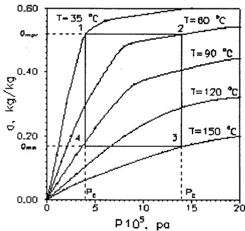
Figure 2. The sorption isotherms for "Busofit"/ammonia are shown on Figure 2.
