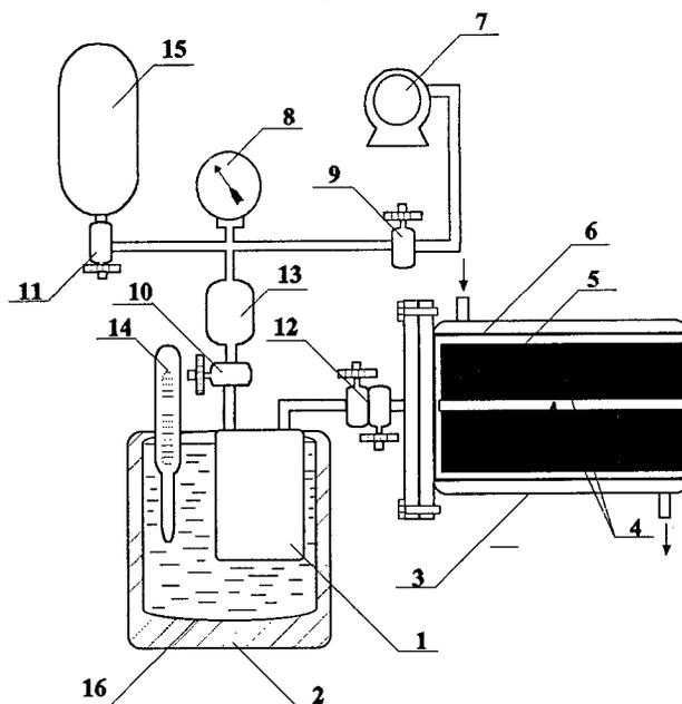
**Figure 1.** The experimental set-up № 1: 1 – evaporator/condenser; 2 – thermal insulation of the thermostat; 3 – heat exchanger; 4 – thermocouples; 5 – sorbent bed; 6 – adsorber; 7 – vacuum pump; 8 – pressure gauge; 9-12 – valves; 13 – control volume; 14 – thermometer; 15 – ammonia vessel; 16 – thermostat.
