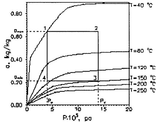
Figure 3. The sorption isotherms for "Busofit"-CaCl<sub>2</sub>/ammonia are presented.
