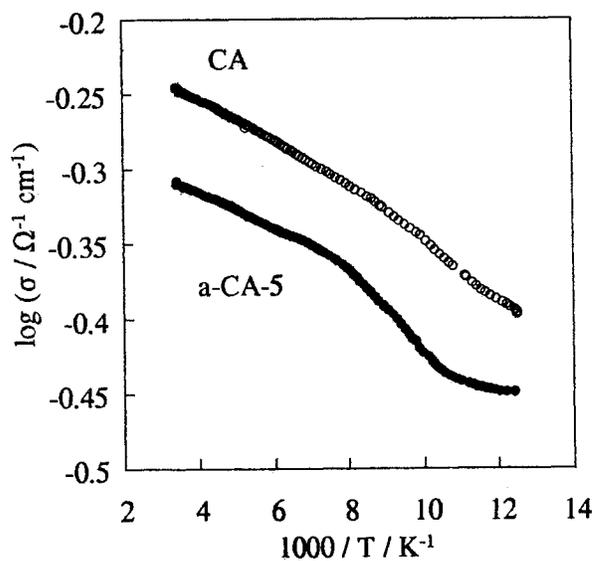
Figure 2. The  $T^{-1/3}$  dependence of dc electrical conductivity of carbon aerogels. (open circle), CA; (closed circle), a-CA-5.
