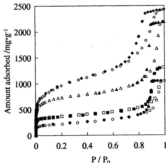
Figure 1. Adsorption isotherms of nitrogen at 77K on activated carbon aerogels. Solid symbols denote desorption. (circle), CA; (square), a-CA-1; (triangle), a-CA-5; (diamond), a-CA-7.
